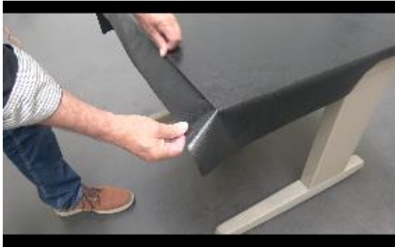
Rub one side from top to bottom.
