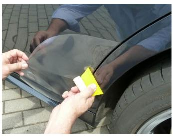
In case of dry wrapping, it is easier to fold the film around the edges afterwards. When dry wrapping, you may see some rubbing stripes in the glue afterwards. These stripes will automatically disappear after some time.
