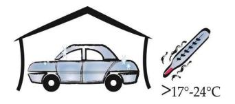
The ideal environment for wrapping a vehicle is a well illuminated, dust-free environment with a constant temperature between 17 and 24°C.
