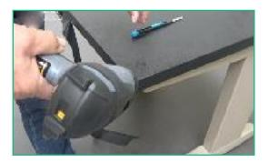
Use a heat gun at 350°C and firmly apply pressure to all edges.
