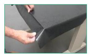
Apply pressure to the vertical sides in a downwards direction.
